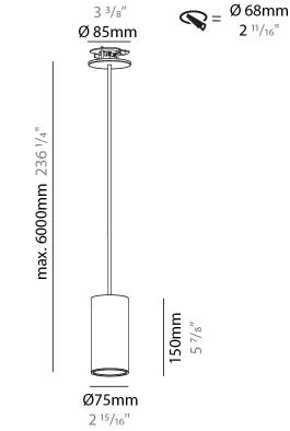
Driver Type: Constant Current - Universal Driver Class: Class 2 Housing: ENCP3 w/Quick Connect Input Voltage (V): 120 - 277 Constant Current (MA): 500 LED Number of LEDs: 1 Color Temperature (°K): 2700 / 3000 / 4000 Max. Delivered Lumen (lm): 923 CRI: >90 CRI Lamp Life (hrs): 50000 Upon Request: \*\*\*3500K available in minimum quantities (larger quantities upon request) Reflector°: 18 / 36 / 52
